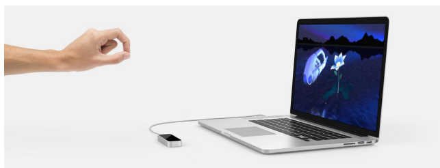
Figure 1: Leap Motion Usage. The small object in the middle is Leap Motion Controller connecting to the Mac on the right. Hand on top of the Leap Motion is tracked and interacted with virtual objects.
